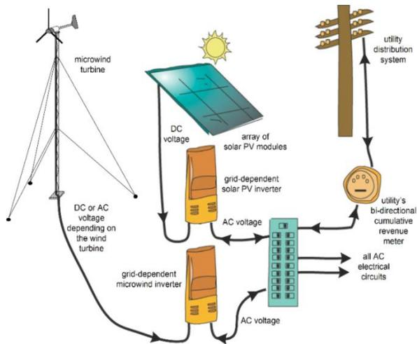
Figure 1. Typical wiring connections for a grid-connected micro wind and solar PV system. (Source: Modified from an unknown source. Gratefully included in this document.)
