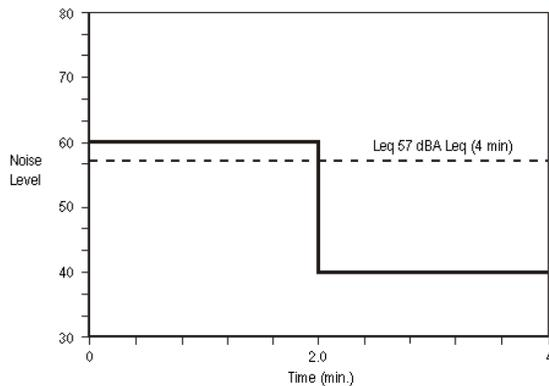
Figure 3 - Illustration of  $L_{eq}$  concept
